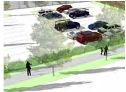
Provide a visual buffer where a parking lot abuts a public sidewalk.
